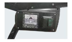
Interactive instrument: The instrument adopts LCD display with four interactive buttons, and has one CAN bus communication function. The communication protocol is compatible with CANopen and SAE |1939 standards.
