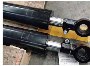
Tilt cylinder piston rod adopts 5-7t
